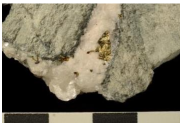
Figure 2: Vein with chalcopyrite (brass colour) a copper mineral, surrounded by quartz (white) hosted by a grey limestone rock. FOV 4 cm. Photo G. Solferino.
