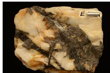
Figure 3: Wolframite (dark grey-black) a tungsten mineral in a quartz vein (white mineral). FOV 10 cm. Photo G. Solferino.
