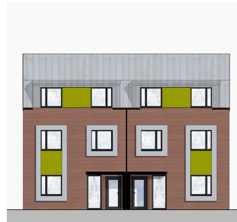
Option C • Red brick • Seamed metal roof • Mansard dormers • Polyester powder coated enamel panels between windows to College colour palette
