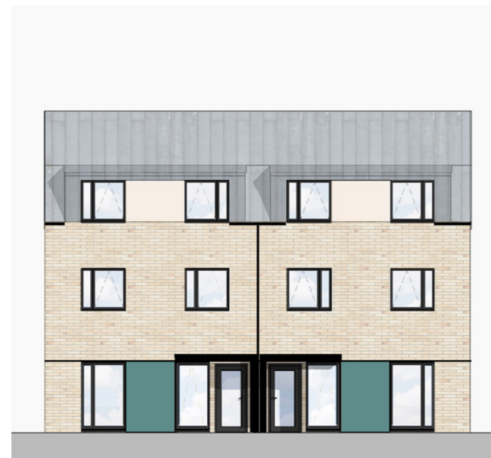
Option B • Seamed metal roof • Mansard dormers • Polyester powder coated enamel panels between windows to College colour palette
