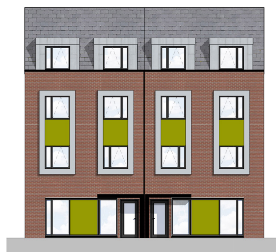
Option F • Red brick • Tiled roof • Seamed metal dormers • Polyester powder coated enamel panels between windows to College colour palette • Frame to upper storey windows seamed metal to match dormers
