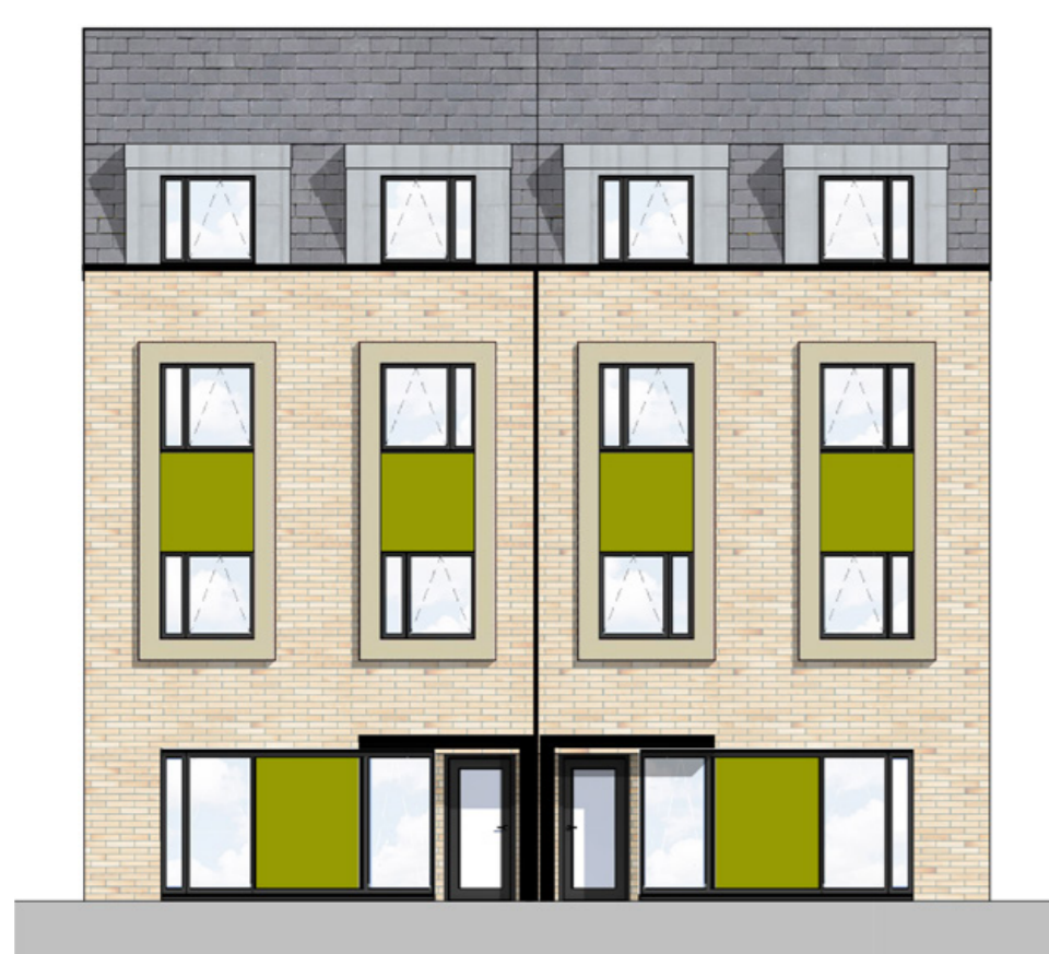
Option E • Buff brick • Tiled roof • Seamed metal dormers • Frame to upper storey windows reconstituted stone or similar
