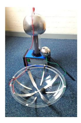
*repulsion* and gives the ball a push along. When it rolls over a grounded strip, the ball becomes *neutralized* and loses its charge. But it doesn't lose its *momentum* and keeps rolling around the bowl. The next time it comes across a charged strip, it picks up the charge again, gets repelled in the same direction as before and once again gets a little kick along. Every time the ball crosses a charged strip it gets *accelerated*.
